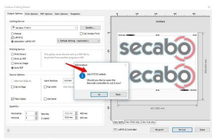
Open the "Lapos Q controller" in the vinyl spooler.
